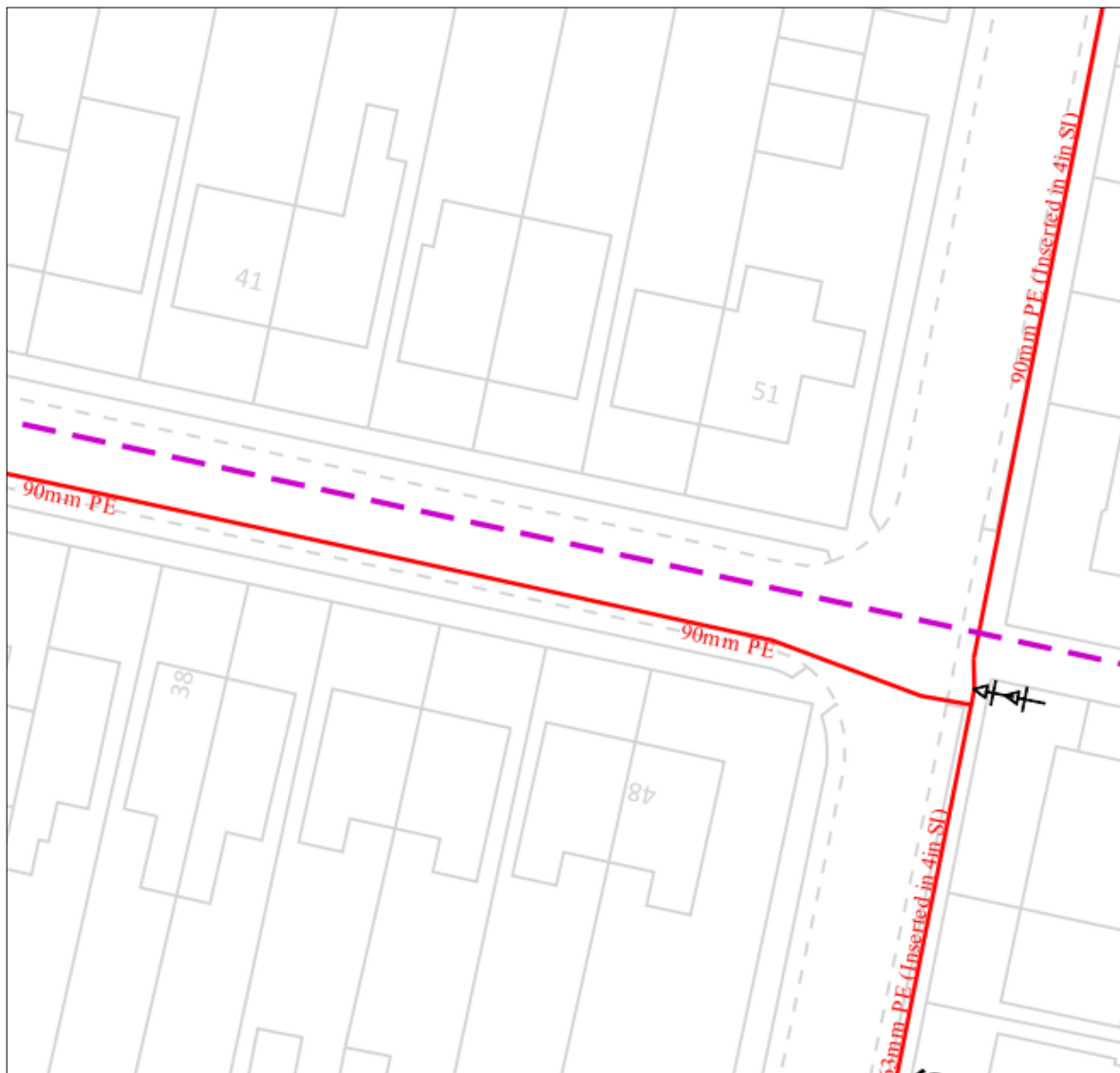
Figure 5.15.4 – Existing underground 90mm PE low pressure gas main in Moira Drive
